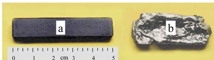
Figure 4 Macroscopic appearance of parent mesophase (a) before and (b) after sintering to 1000°C.
